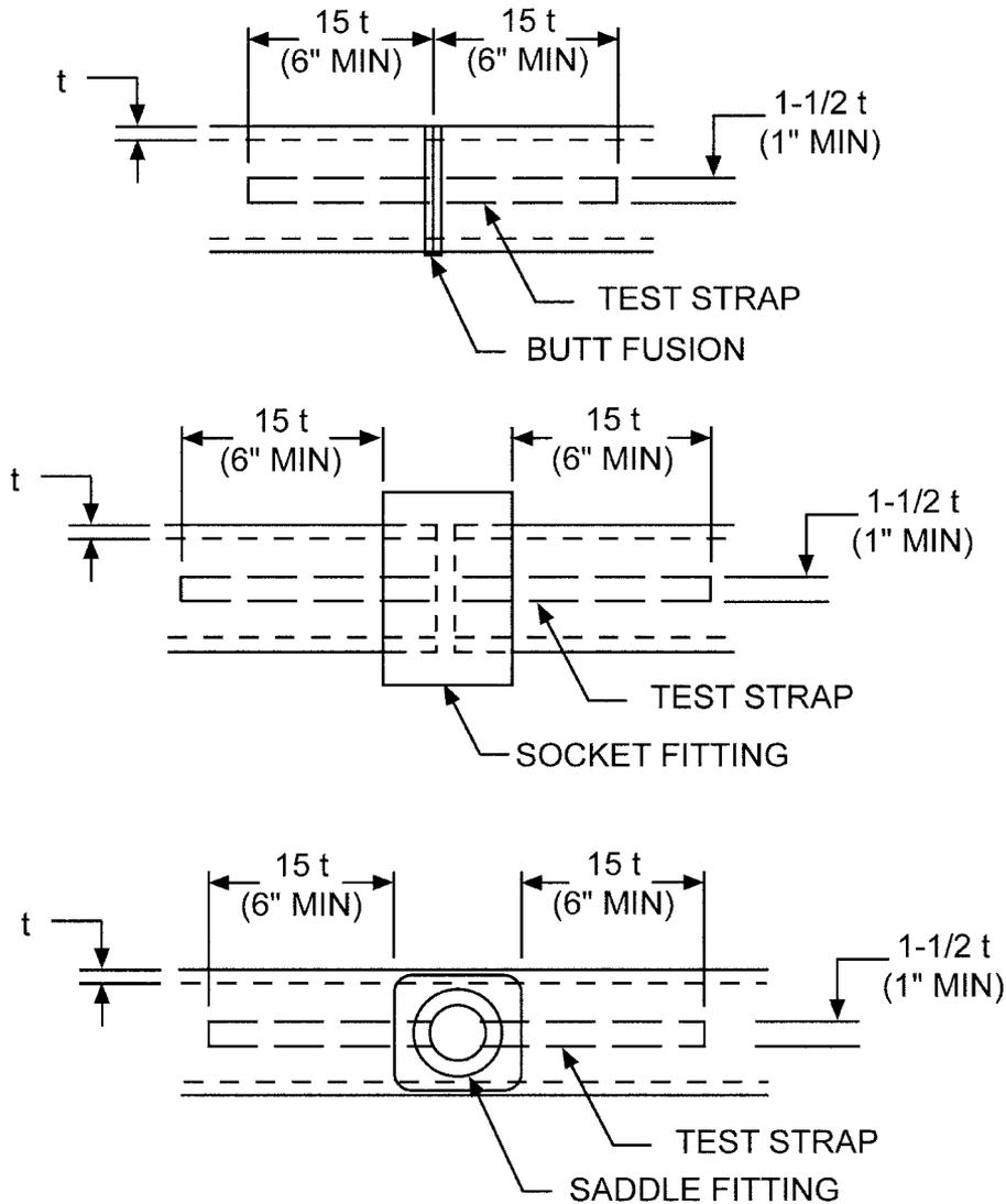
FIG. X4.1 Bent Strap Test Specimen
