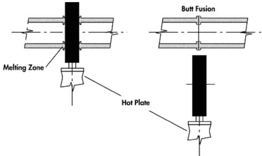
FIG. 2 Butt Fusion
