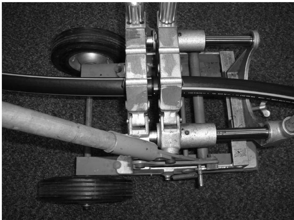
FIG. X2.15 Coiled Pipe Installation in Fusion Machine
