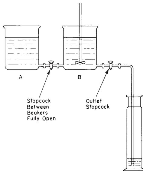
FIG. X2.2 Apparatus for Gradient Tube Preparation
